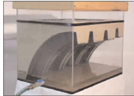
Figure 6: Quick4 Standard chamber during the introduction of water
