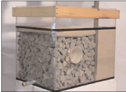
Figure 3: Aggregate test box with rigid plastic divider in place
