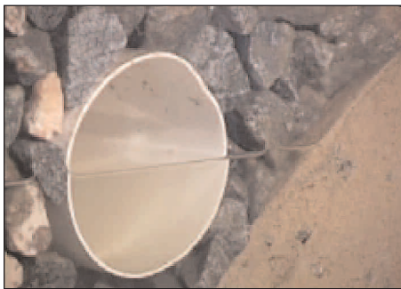
Figure 5: Close up of sand infiltration after introduction of water
