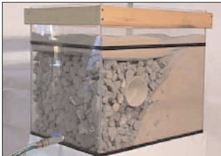
Figure 4: Aggregate test box with rigid plastic divider removed
